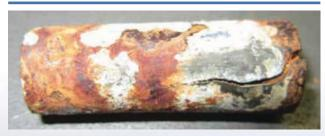
FIGURE 2: THIS COILED PIN WAS FINISHED WITH A LIGHT DUTY ZINC PLATING AND SUBSEQUENT CHROMATE DIP. THE FINISH WAS RATED FOR 48 HOURS TO 'RED' CORROSION PROTECTION. LEAVING THIS ITEM IN SALT SPRAY FOR 200 HOURS HAS RESULTED IN SIGNIFICANT RED RUST THOUGH SOME ZINC AND WHITE CORROSION REMAIN. WHERE ZINC IS PRESENT ON THE SURFACE, THE PART REMAINS FREE OF RED RUST DESPITE THE SEVERITY OF ATTACK IN ADJACENT AREAS.
