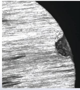
FIGURE 10: CROSS SECTION OF PIT SHOWN IN FIGURE 9 DEMONSTRATING IMPACT ON CROSS-SECTIONAL AREA AND REDUCTION IN STRENGTH.
