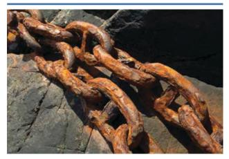
FIGURE 1. RUSTING CHAIN DEMONSTRATES MATERIAL LOSS DUE TO RUST OR GENERAL ATTACK.
