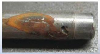
FIGURE 9: PITTING WITH RELATED STAINING ON A 410 STAINLESS STEEL SOLID PIN.
