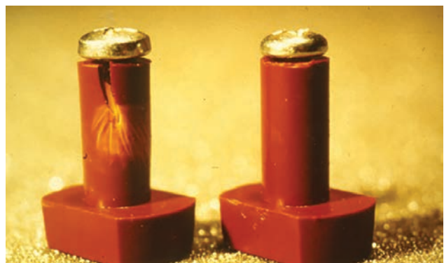
FIGURE 1: TYPE AB SCREW ON LEFT AND SCREW THREAD FOR PLASTIC APPLICATIONS ON RIGHT
