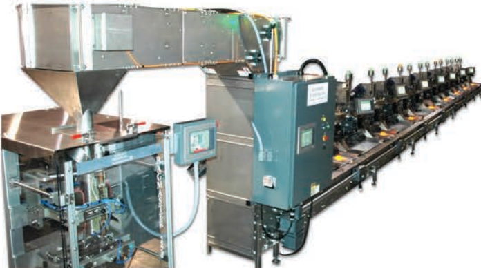
Kit Line with Batchmaster® IV Counters, Conveyor & Bagmaster® Bagger
