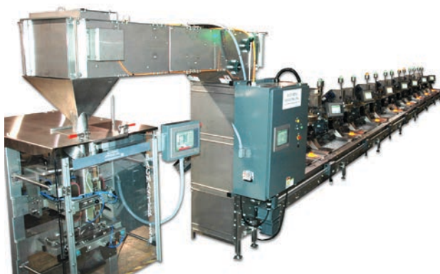
FULLY INTEGRATED TURNKEY PACKAGING SYSTEM WITH BATCHMASTER® IV COUNTERS, CONVEYOR, AND BAGMASTER® BAGGER FROM BATCHING SYSTEMS, INC.
