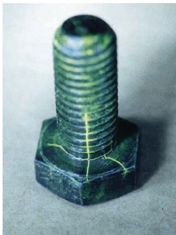
FIGURE 1 - A HEX CAP SCREW WITH QUENCH CRACKS OPEN TO THE SURFACE. THE CRACKS ARE SHOWN IN FLUORESCENT GREEN UTILIZING MAGNETIC PARTICLE TESTING
