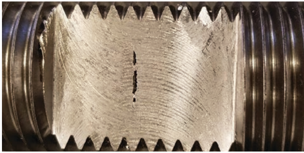
FIGURE 3 - A CUTAWAY SECTION OF A FULLY THREADED STUD SHOWING A VOID OF MATERIAL KNOWN AS A BURST
